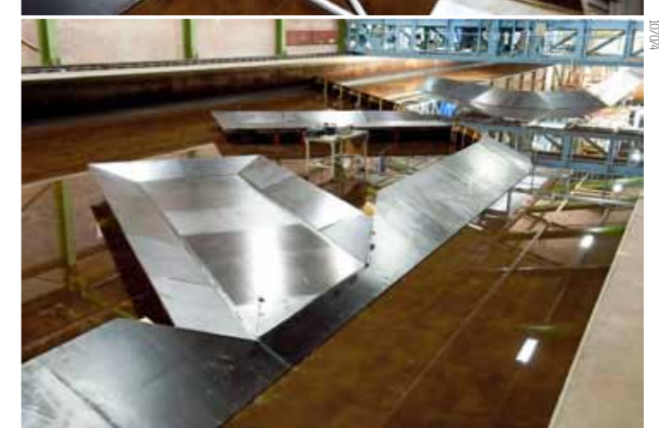
Harbours being built-up: construction of main waterway, secondary shipping channel, two barge docks and final test set-up
